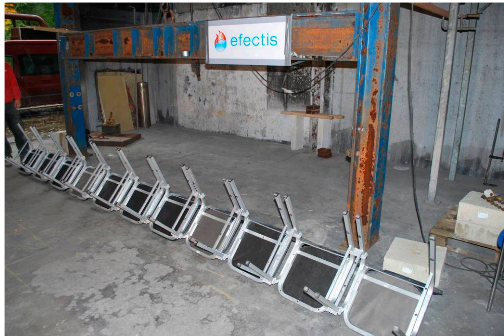
Photo 4: push/pull test in action
