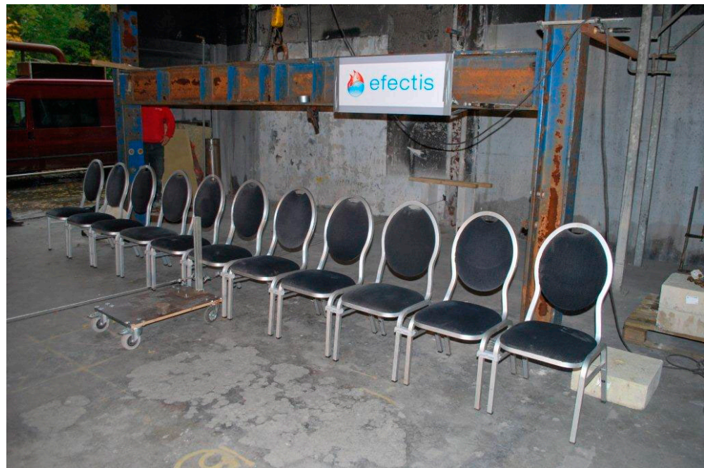
Photo 3: row-movement test in action
