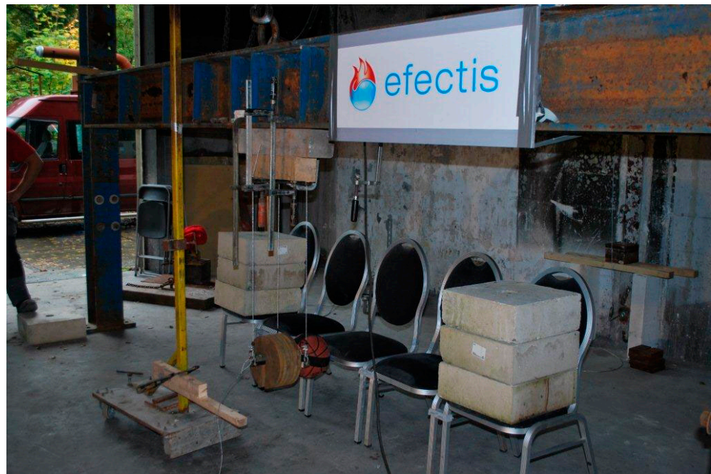
Photo 5: Horizontal impact test in action
