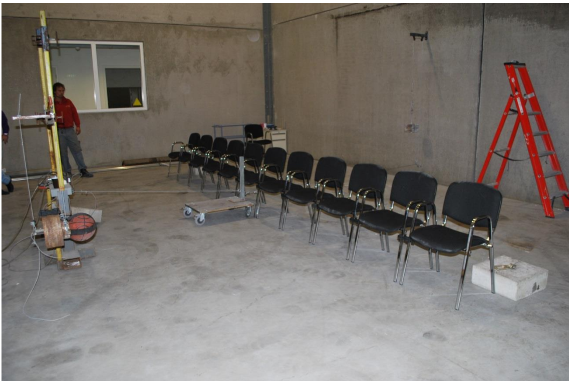
Photo 3: row-movement test in action
