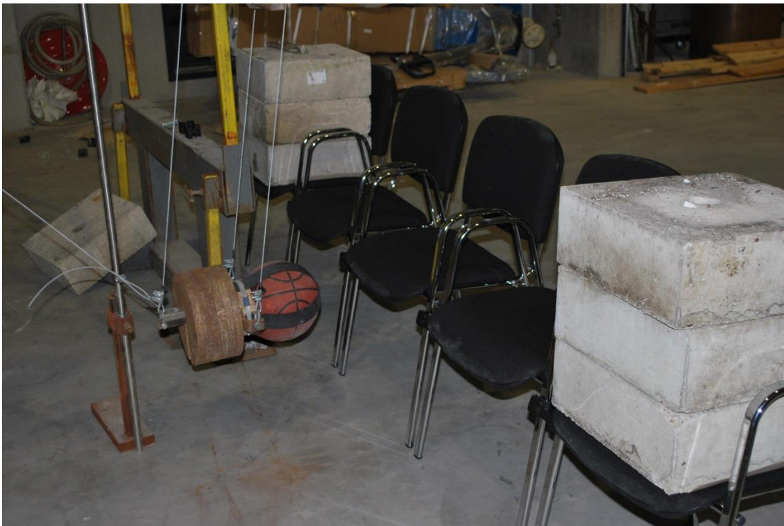
Photo 5: Horizontal impact test in action
